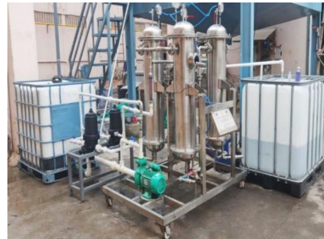
30 KLD pilot plant for feasibility field trials( at JSC, Jodhpur (>5,00000L))
